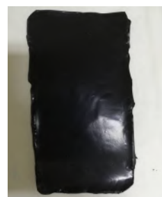
Figure 1: Conducting Polymer Composite which could be readily prepared in the form of thin film suitable for SPE applications.
