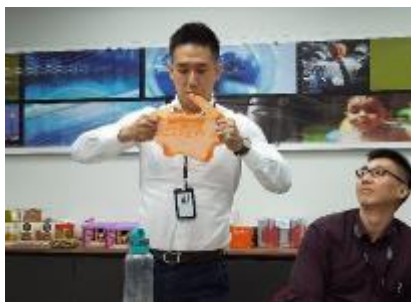
Figure 1: Mr. Chan Yian Kit of TA Instruments is testing the strength of plastic bag with different molecular alignments
