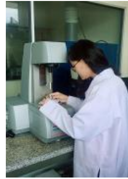
Figure 2: Ms. Wong Kai Yi uses the newly purchased rheometer from Anton Paar installed in TAR UC to measure the viscosity and study the rheological behavior of polyurethane.
