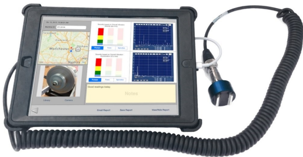
Figure 1 : Example of a portable vibration measurement system (Credits to Motionics)
