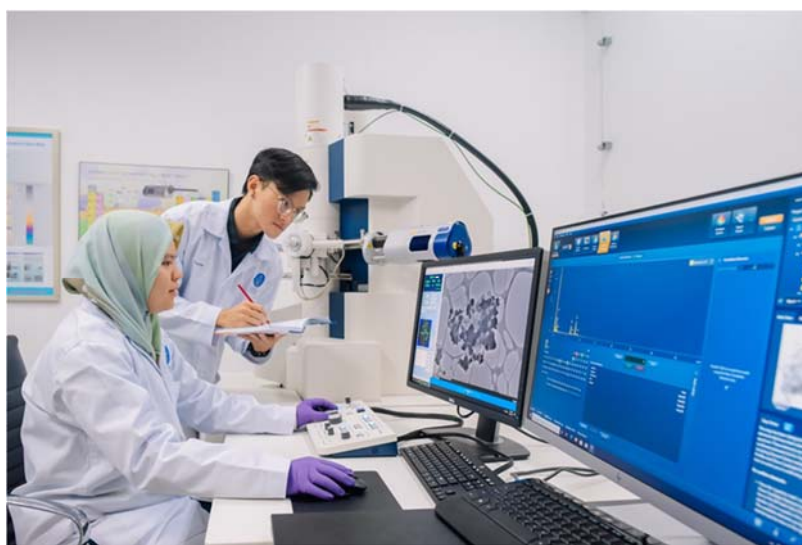
Figure 3 The transmission electron microscope, one of the state-of-the-art analytical instruments at UTP, produces a high-resolution imaging technique that yields information on the morphology, crystal phase, crystal structure and defects
