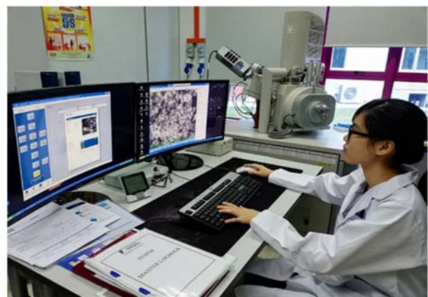
Figure 3 A materials engineering graduate student undergoing practical training with Field Emission Scanning Electron Microscope (FESEM) and Energy Dispersive X-ray (EDX) analysis at the University of Nottingham Malaysia
