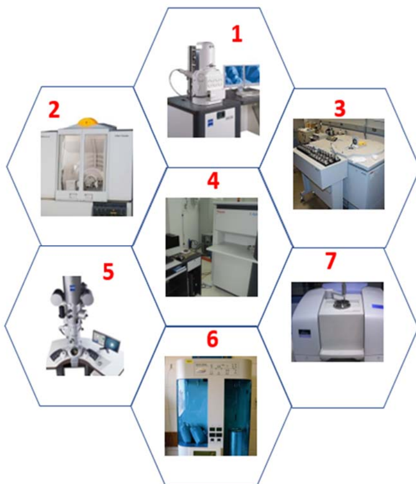
Figure 1 Analytical equipment facilities supporting the Materials Engineering programme 1. Scanning Electron Microscopy (SEM): For the determination of surface morphology 2. X-ray Diffraction (XRD): For determination of structure and purity 3. X-ray Fluorescence (XRF): For determination of elemental composition and purity 4. X-ray Photoelectron Spectroscopy (XPS): For determination of surface chemistry 5. Transmission Electron Microscopy (TEM): For determination of average particle size 6. Brunauer-Emmett-Teller (BET): For the determination of specific surface area 7. Fourier Transform Infra-Red (FTIR): For the determination of chemical composition
