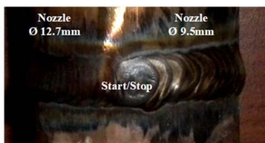
Figure 2: Sample no. 3 weld bead geometry
