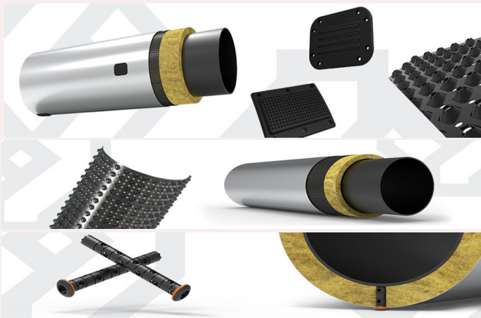
Figure 2: CUI insulation ventilation drains accessories to promote airflow along the insulation system – Drying out wet insulation.
