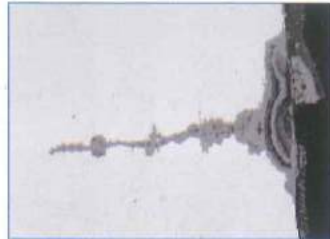
Fig 8: Backscattered image of a corrosion fatigue crack in mild steel
