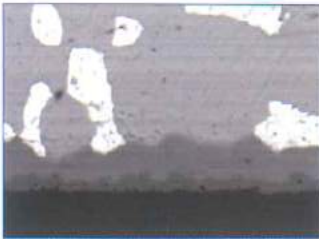
Fig 7: Backscattered electron image of the interface of a failed electronic joint
