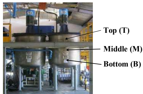
Figure 1 Sampling of samples was done from the Top (T), Middle (M) and Bottom (B) of the mixing tanks
