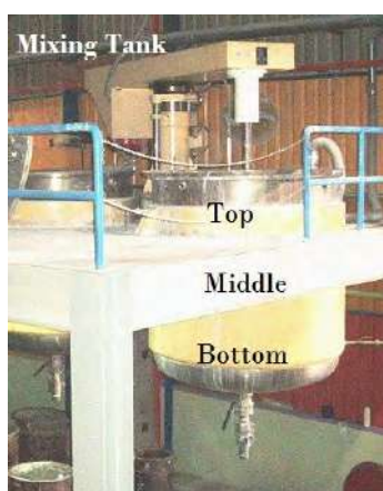
Figure 1 Mixing tank of the immediate material (e.g. epoxy or hardener)
